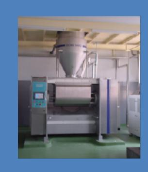
Double arm mixer Capacity – 190kg/batch
