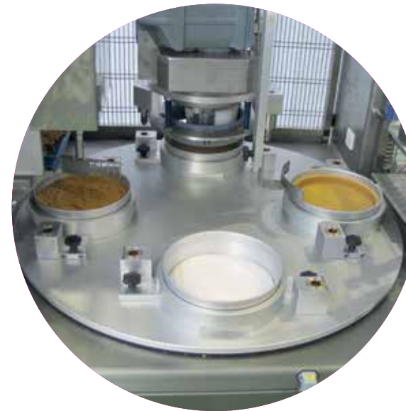
Tartomatic turntable equipped with cheesecake base forming tools.
