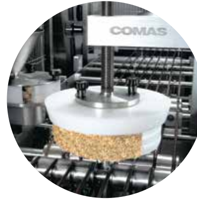
Dry granular product coater station
