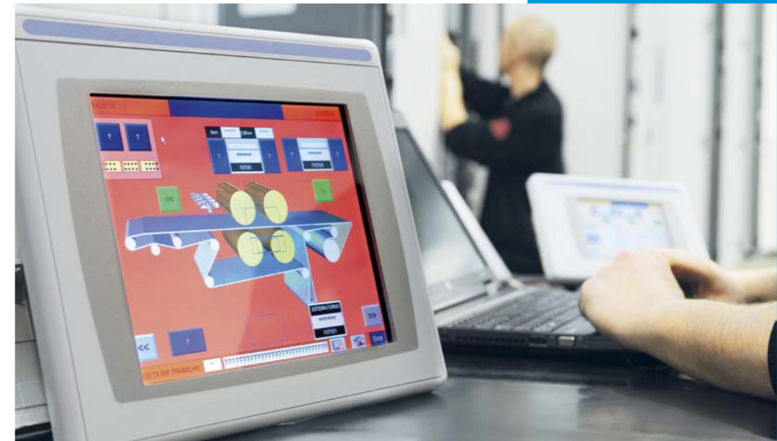
Automatic dough sheet loop control system GEA Imaforni has developed an automated control system to ensure a constant tension in the dough sheet as it enters the nip of the final gauge roll. No manual intervention is required, and customers can be confident of improved consistency and quality of the final product.
