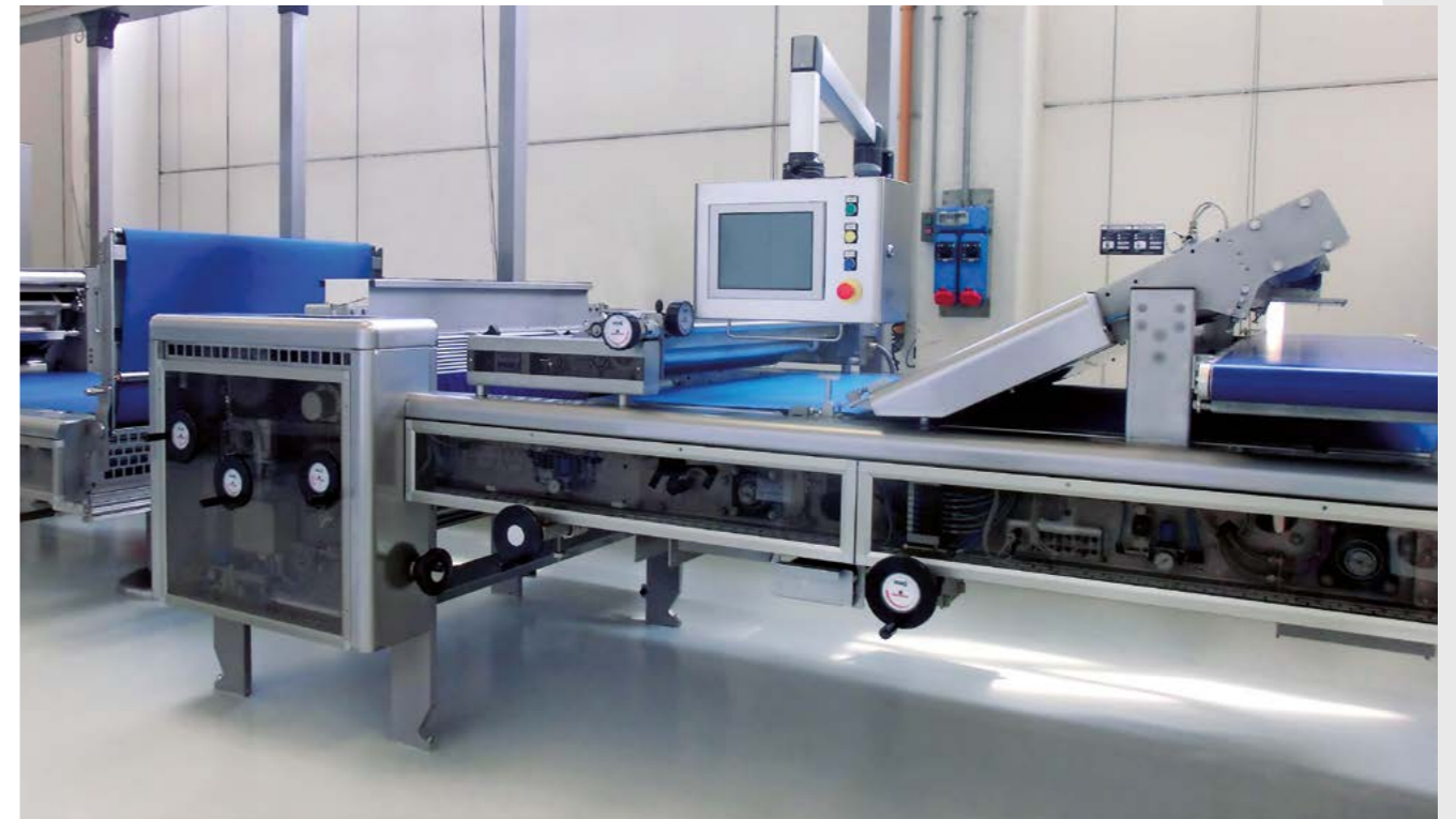
Rotary cutter/rotary moulder machine equipped with a washover device
