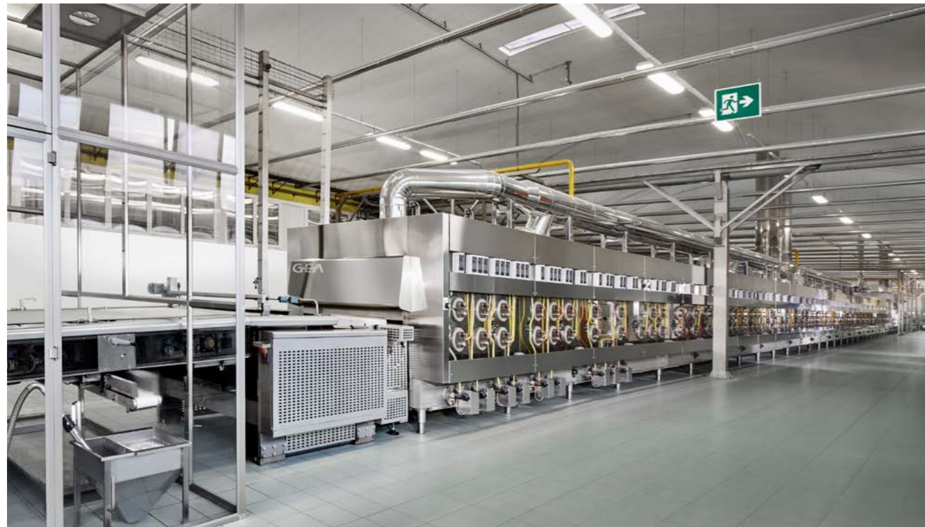
Hybrid oven - Direct gas fired zone
