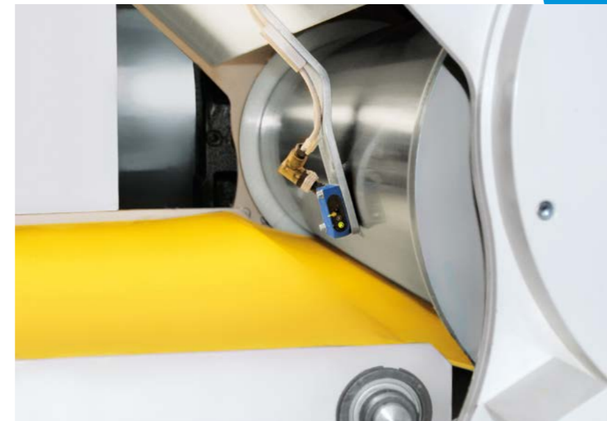
Automatic dough sheet loop control system GEA Imaforni has developed an automated control system to ensure a constant tension in the dough sheet as it enters the nip of the final gauge roll. No manual intervention is required, and customers can be confident of improved consistency and quality of the final product.
