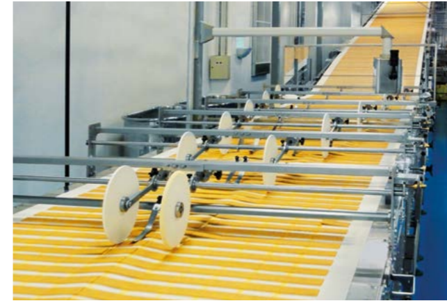
Top rollers gently break the strips of soda crackers to create single portions.
