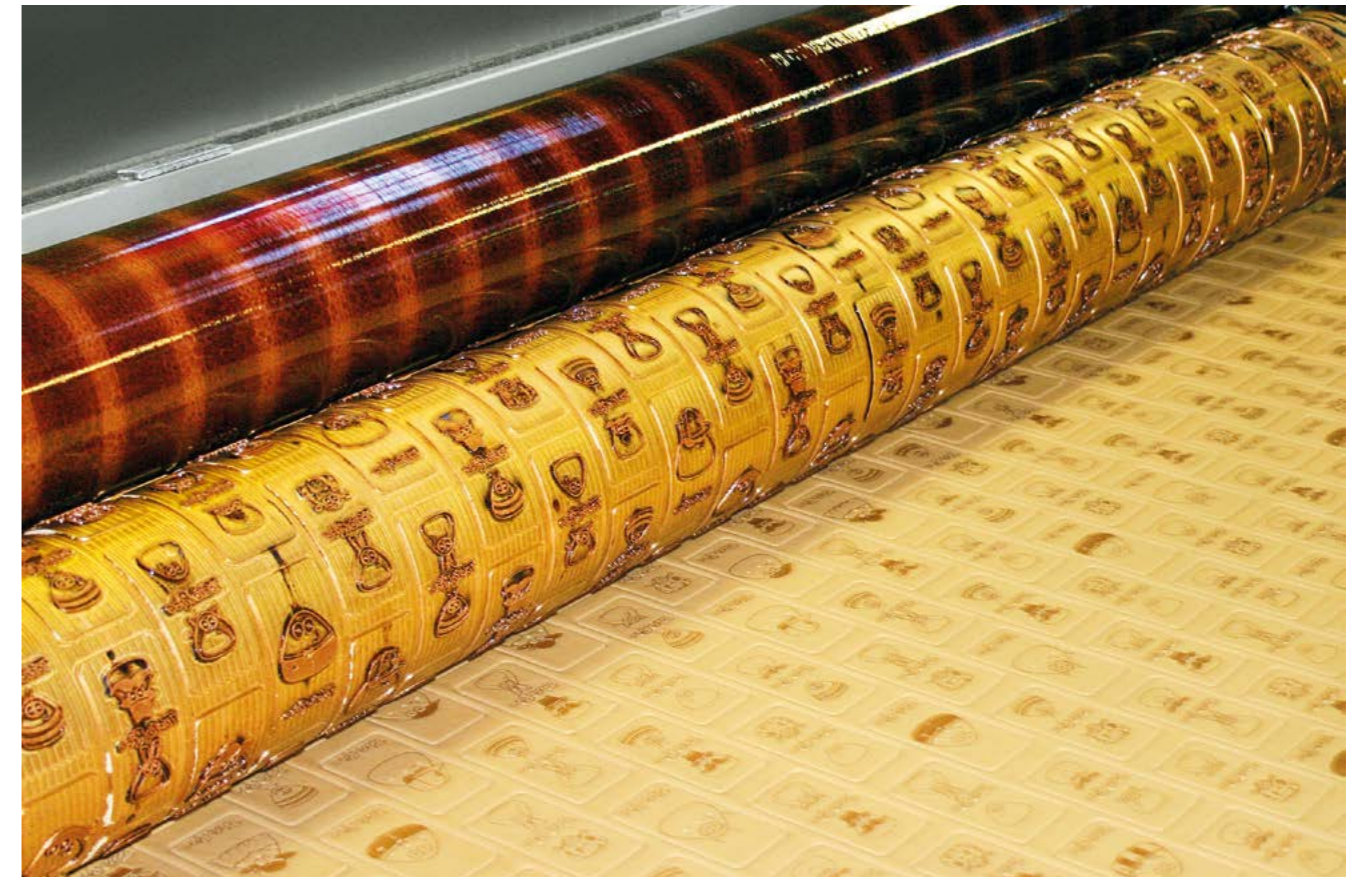
Ink printer installed between the rotary cutter and the scrap pick-up conveyor
