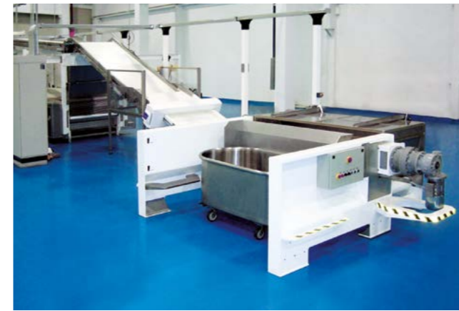
Ground floor tub tilting system
