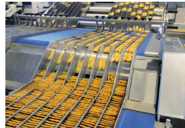
Stainless steel inclined chute aligns the crackers between guides, in advance of a star wheel type stacking system.
