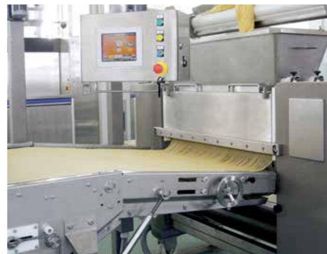
Full width extruder with bread-stick dough ropes
