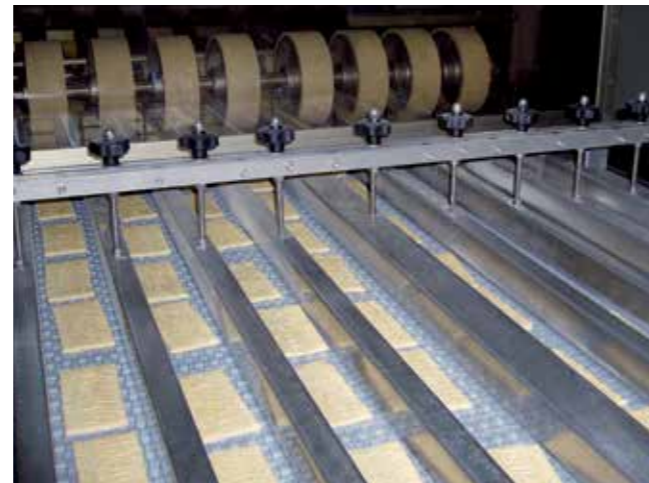
Single pieces are formed after the breaker
