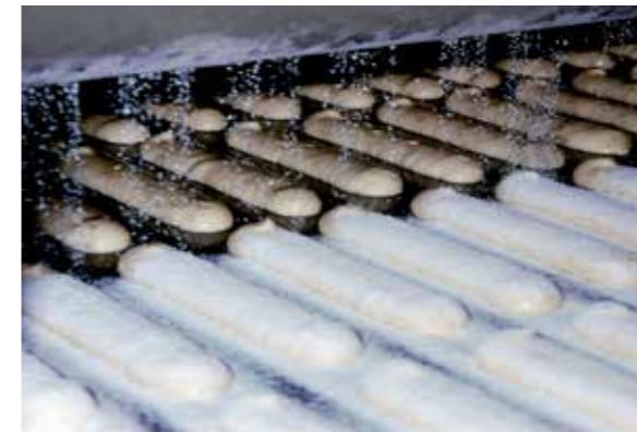
Sugar is immediately sprinkled on top of deposited products on the steel band of the oven.
