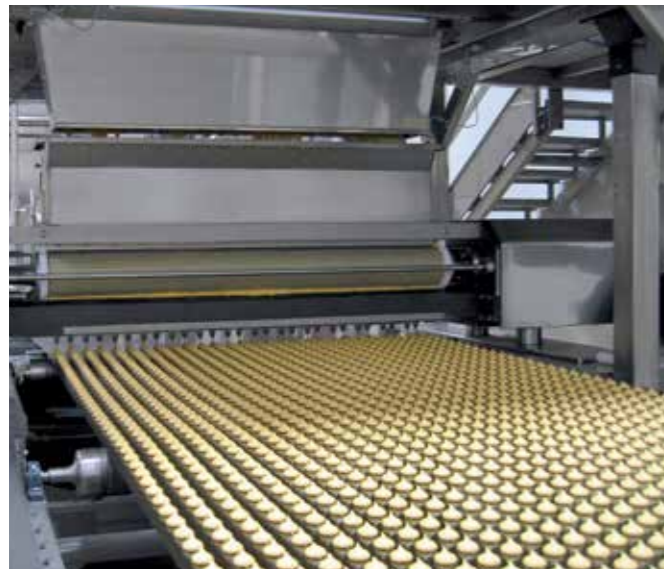
Choux bun batter deposited directly on a 1,500mm wide oven band
