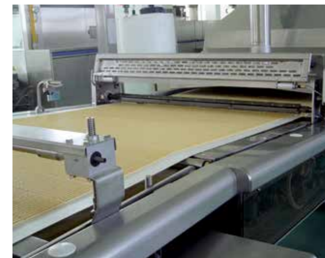
Bread-sticks extruded onto a plastic belt
