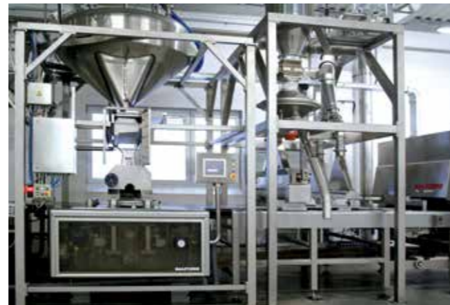
Depositor and a topping unit with integrated recovery and circulation system
