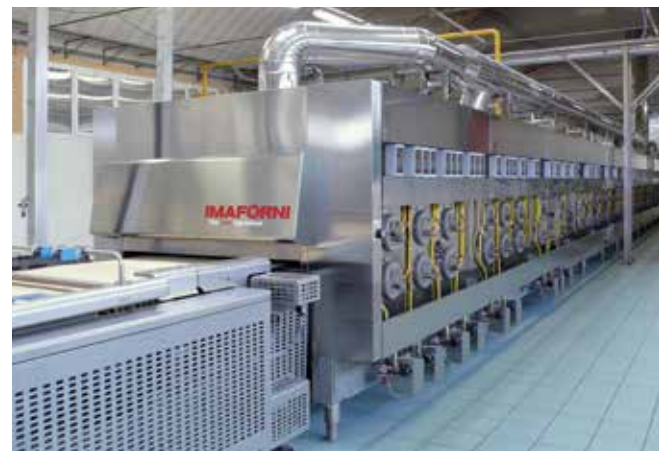
Main exhaust collection duct is connected to the oven heat recovery system
