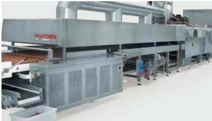
Configuration options include installing a water jet cleaning system for the oven wire mesh conveyor
