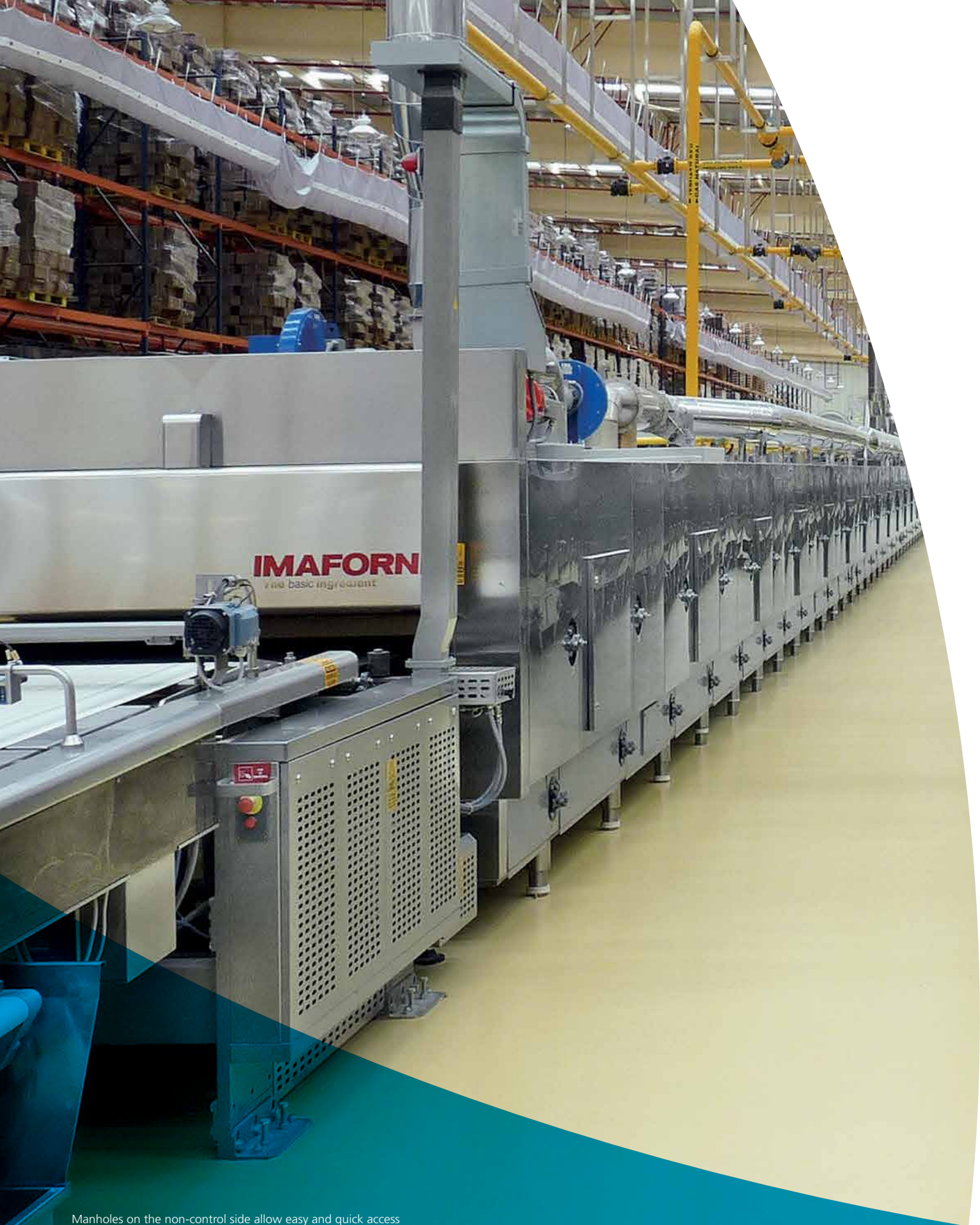
Manholes on the non-control side allow easy and quick access to the baking chamber for cleaning or maintenance purposes
