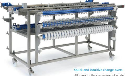
All items for the change-over of products are studied to be removed without tooling. These items are designed for removal and replacement on accurate and repetitive basis by using a series of centering and locking devices that allow a rapid change of product and safe restarts without loss of position. Each set of items is housed on a trolley provided.
