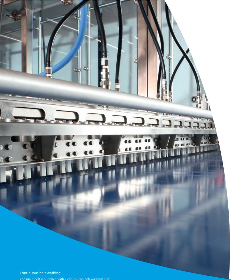
The main belt is supplied with a continuous belt washing and drying system. This system can come equipped for washing with water jets or steam.
