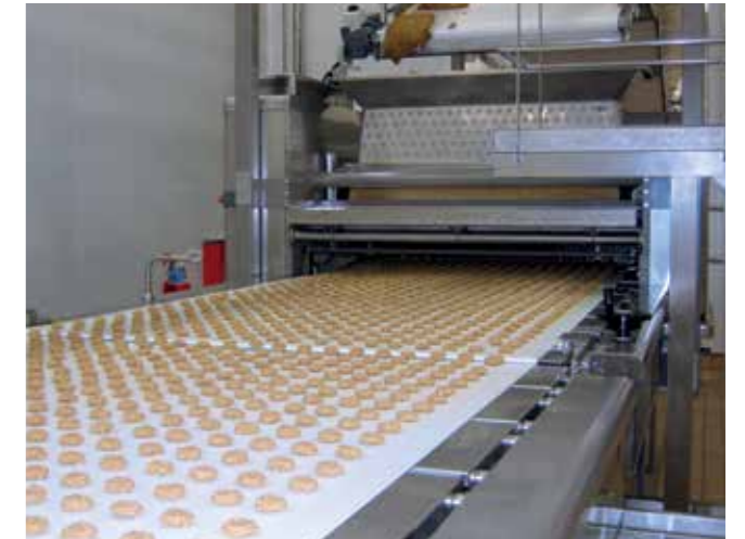
A plain wirecut unit in production
