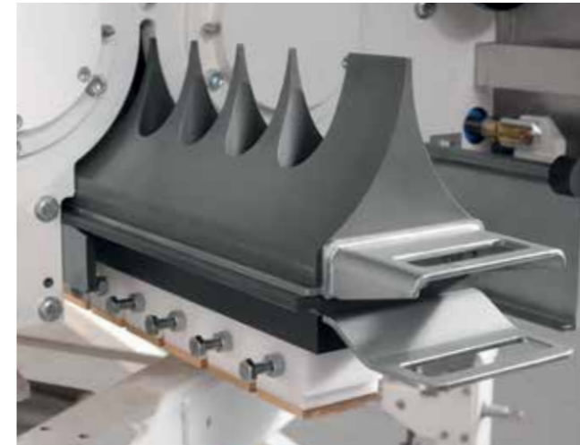
A filler block aids dough distribution and weight control
