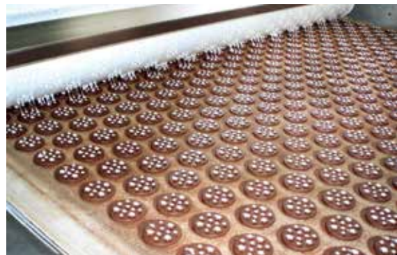
Egg wash unit in operation
