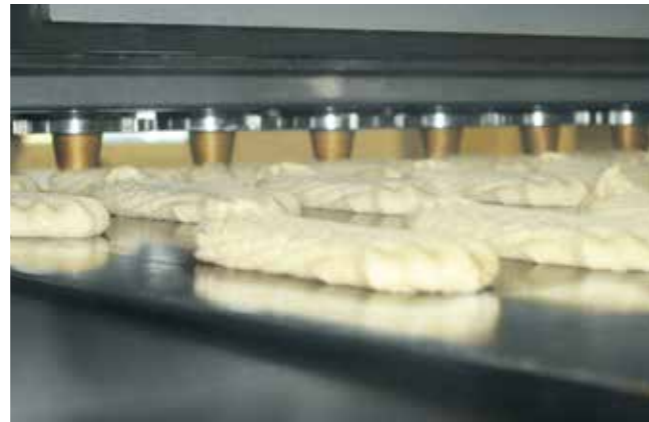
A volumetric pump ensures accurate dosing
